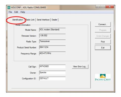
• Go to the Radio Link Tab to configure the radio link settings
